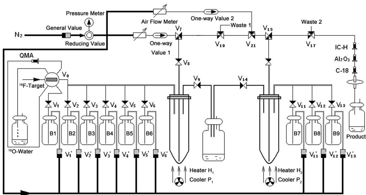
Figure 8: Schematic diagram of the automated synthesis of  $^{18}\text{F}$ -FEL on the PET-MF-2V-I synthesis module.
