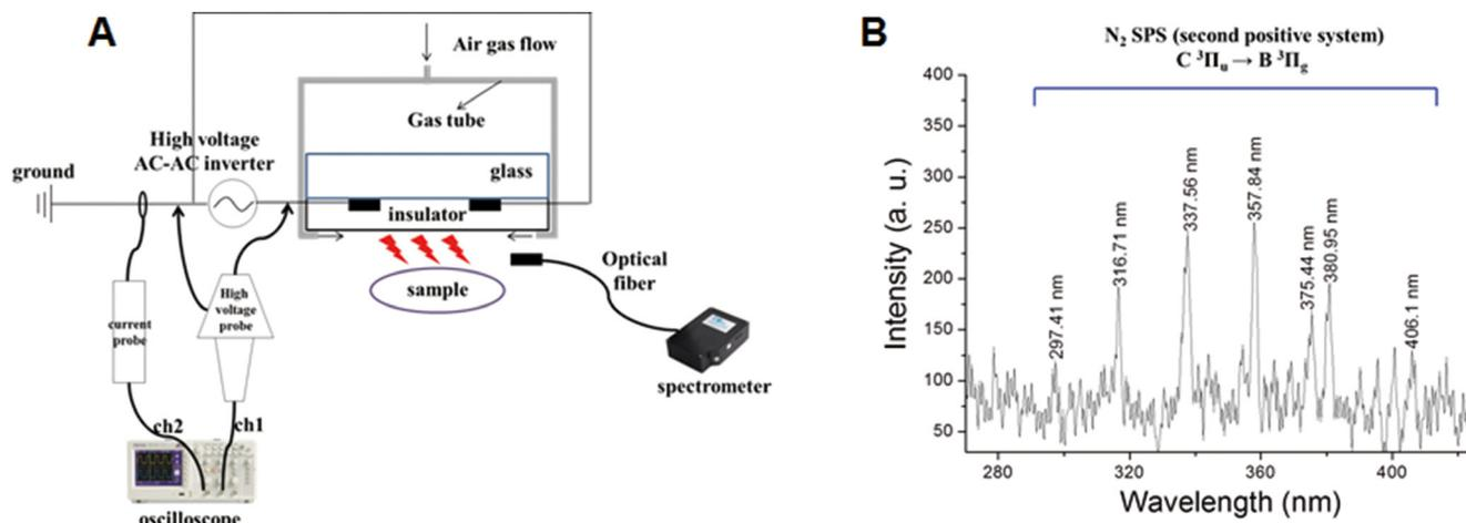
Figure 1: Schematic illustration of NBP device and OES spectrum.
