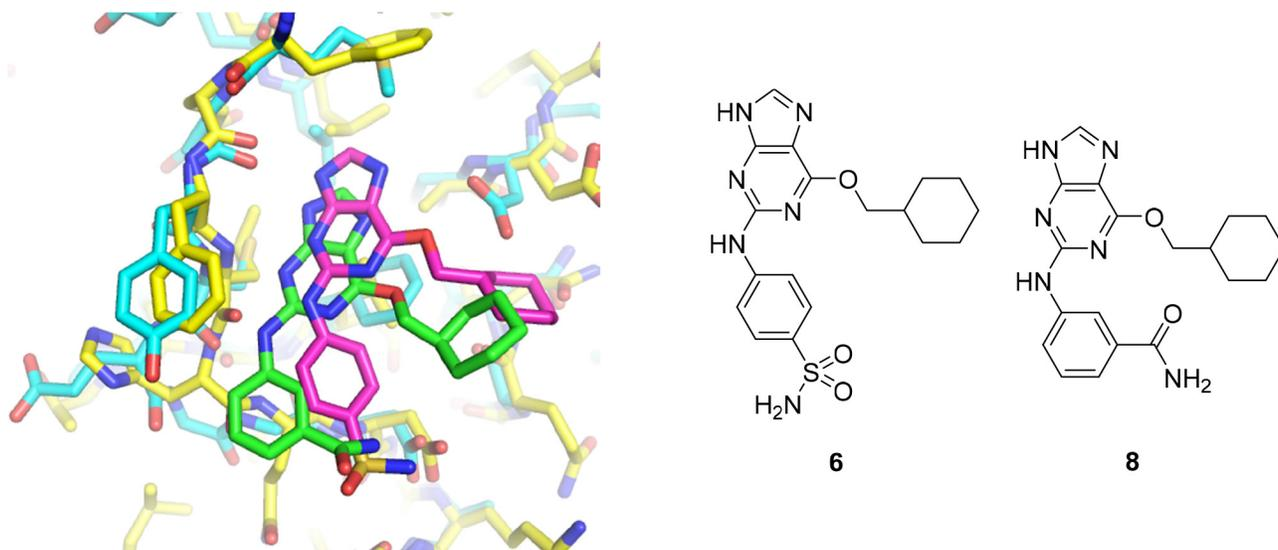
**Figure 2: Structural overlay of 8-T175A-Nek2A complex (green and cyan) and the 6-T160pCDK2-cyclin A (pink and yellow).** Rotation of the 2-arylamino group with respect to the purine is only observed for **6** in CDK2, but not for **8** in Nek2.
