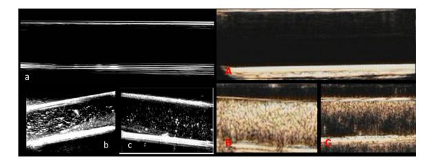
Figure 7: Two-dimensional ultrasonic imaging and ultrasound contrast enhanced imaging of UCAs *in vitro*. Twodimensional ultrasonic images: **a**. a tube filled with degassed aqueous, **b**. SonoVue in degassed aqueous. **c**. NPs in degassed aqueous. Ultrasound contrast enhanced images: **A**. a tube filled with degassed aqueous, **B**. SonoVue in degassed aqueous. **C**. NPs in degassed aqueous.
